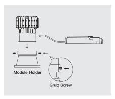
3. Grub screw to tighten between module & module holder and connect module to driver.
